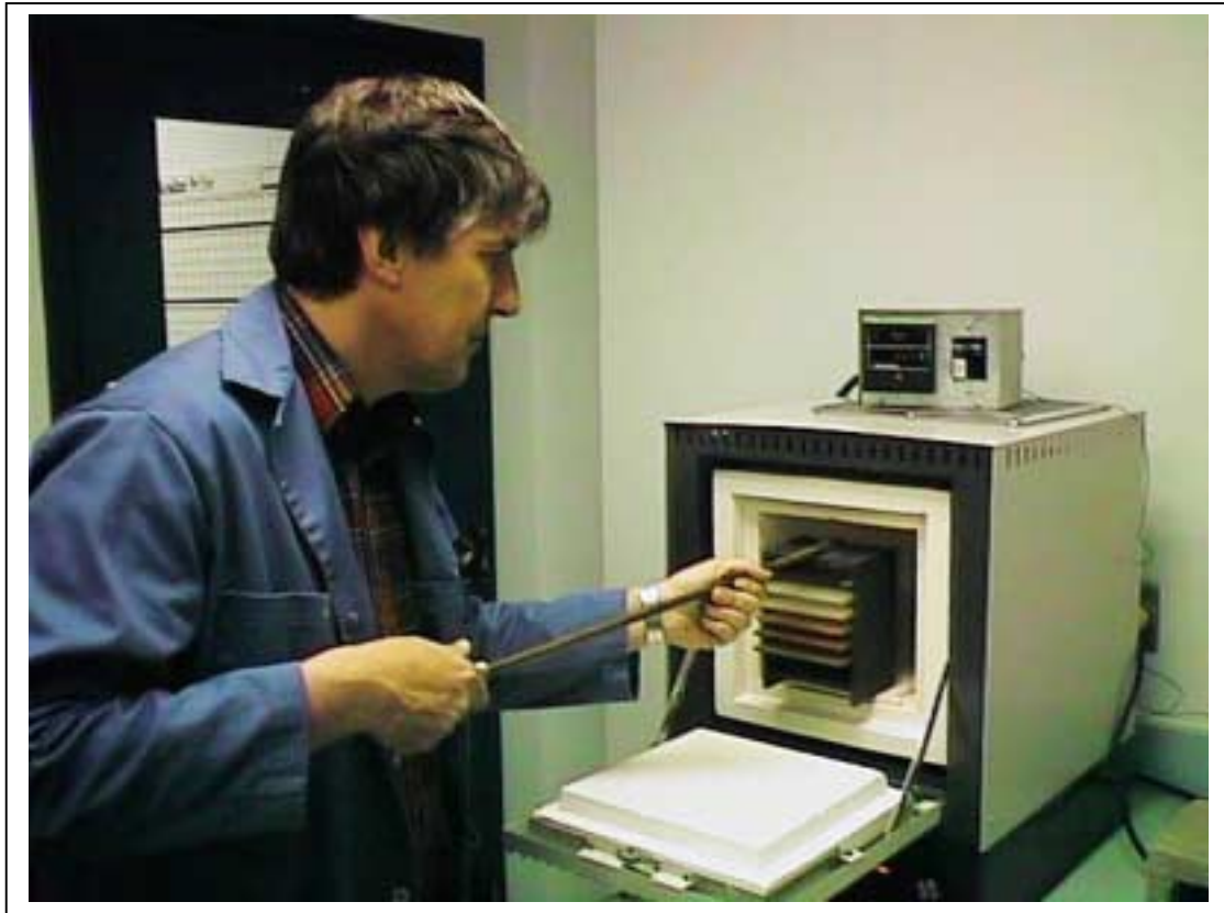
Figure 1. Silver membrane filters being placed in the muffle furnace for RCD analysis.
