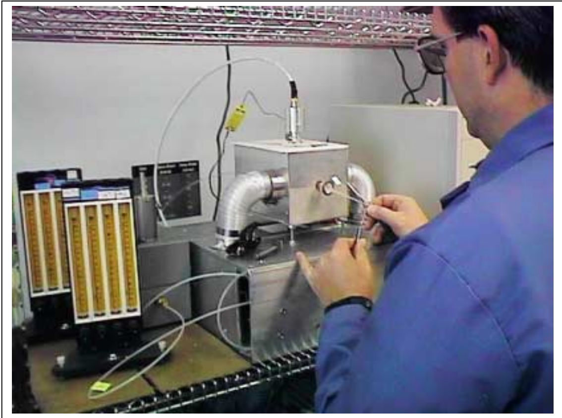
Figure 2. Sample filter cut-out being inserted into the oven for Thermal-Optical analysis.
