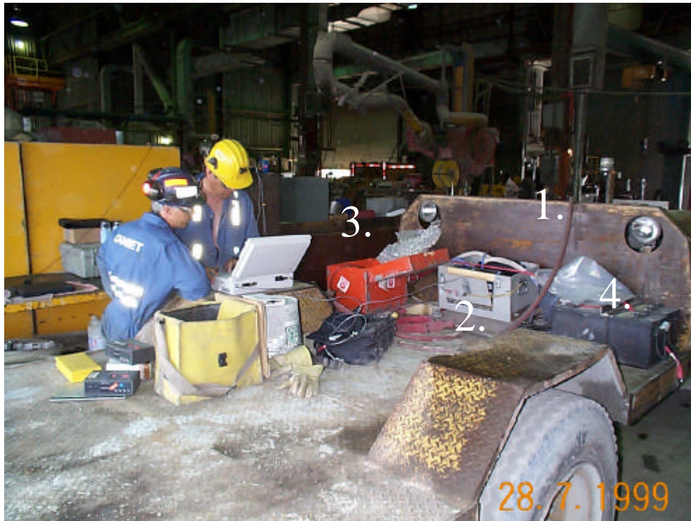
Figure 3. Warehouse truck flat-bed with: 1- heat-traced DPM sampling line, 2- ECOM gas analyzer, 3- DPM sampling box and 4- 24 volt power pack.
