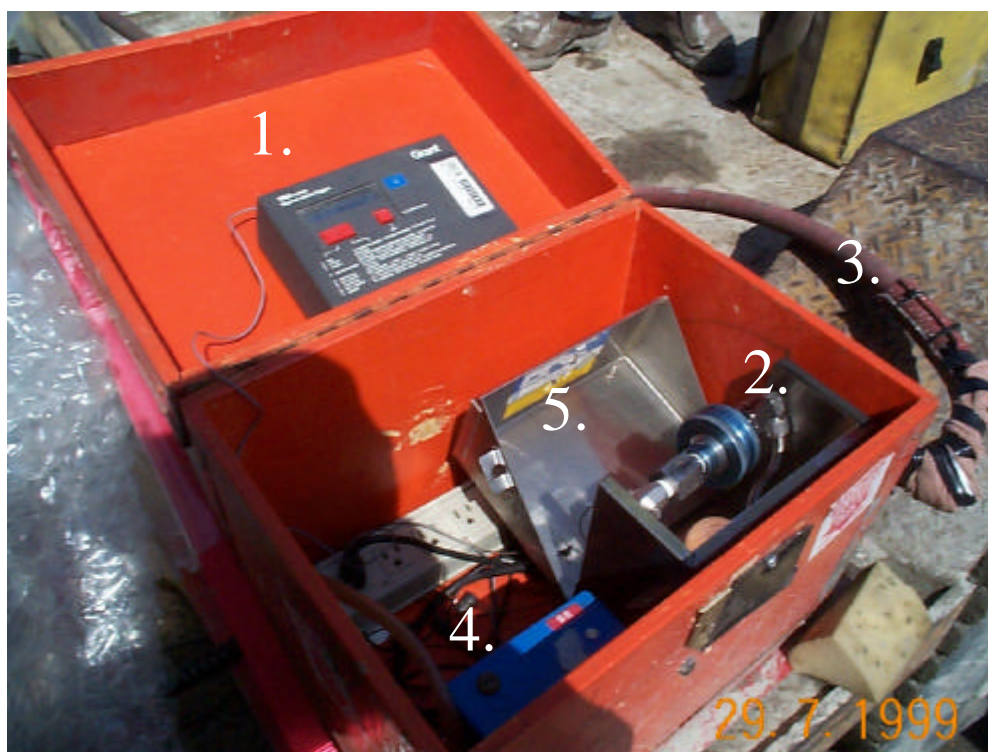
Figure 2. Heat-traced DPM sampling apparatus showing: 1- the data logger (sample temperature), 2- the filter holder, 3- the heat-traced sampling line, 4- the sampling pump and 5- the stainless steel filter assembly enclosure.
