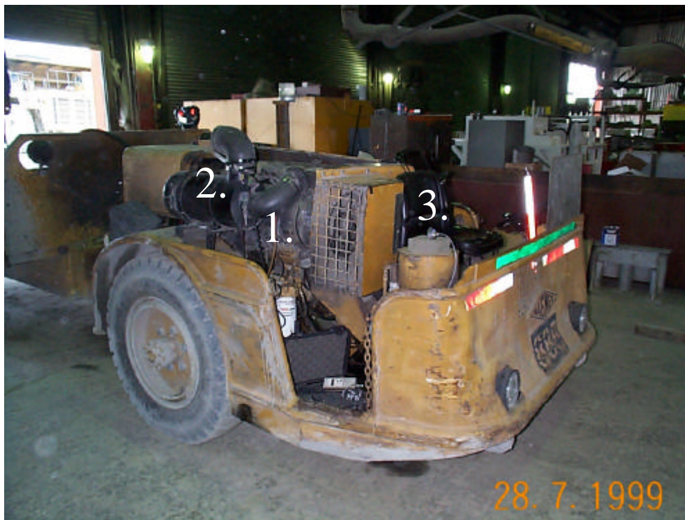
Figure 4. Warehouse truck showing: 1- RPM sampling on fuel injector lines, 2- relative humidity and temperature probe and 3- atmospheric pressure monitor.
