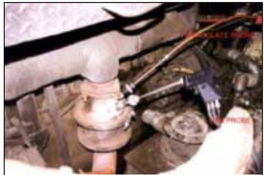
Fig. 7-1 Sampling Undiluted Particulate Matter
