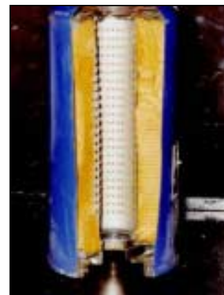
Fig. 8-2 Cut-Away of a Contaminated Fuel Filter
