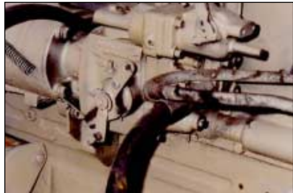
Fig. 8-14 Cummins PT Fuel System
