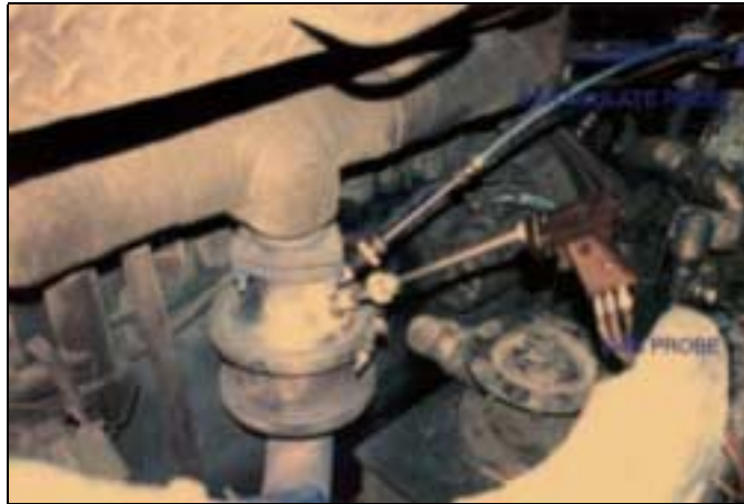
Fig. 5-3 Performing an Emissions Test
