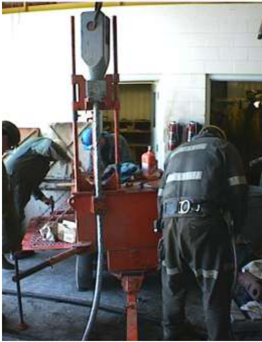
Fig. # 6 - These photos show the concept of holding the socket in line with the rope using a socketing table.
