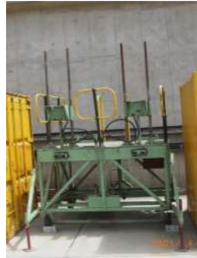
Fig. # 6 - These photos show the concept of holding the socket in line with the rope using a socketing table.
